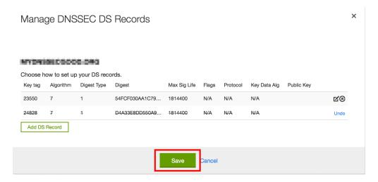
Fig. 15: Remove DS Record Step #3
