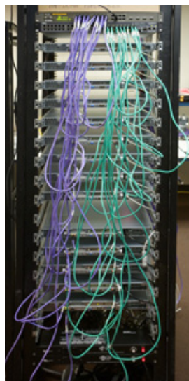
Testbed from the back. Lavender wires (left) are to the Gigabit data network; turquoise wires (right) are to the IPMI network. Power lines run inside a channel built in to the right edge of the rack.
