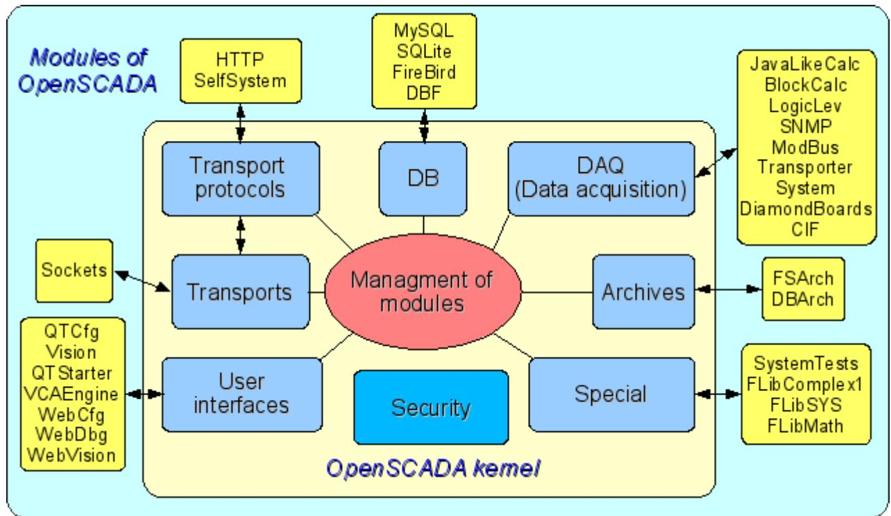
Fig. 1. The block scheme of OpenSCADA system
