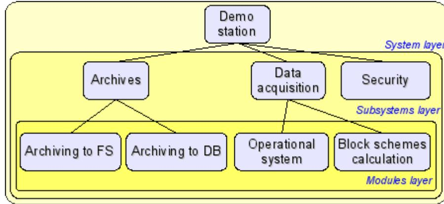
Fig. 2. Hierarchical structure of OpenSCADA.
