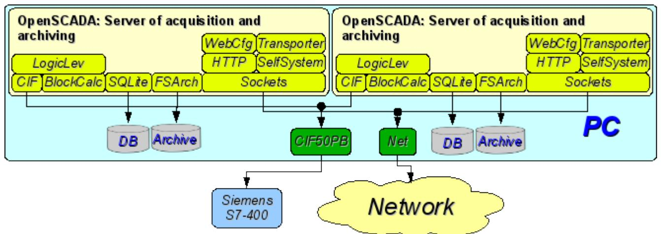
Fig. 3.3. The duplicated server connection on one server.
