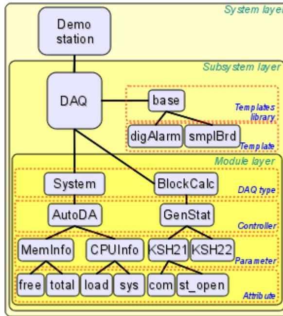
Fig. 4. Hierarchical structure of the data acquisition subsystem.
