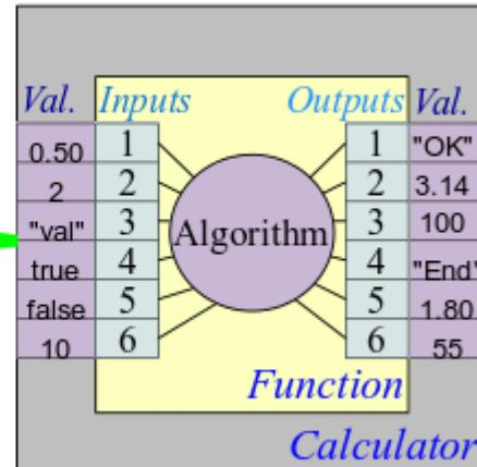
Fig. 7. The basis of the programming area of the OpenSCADA system.
