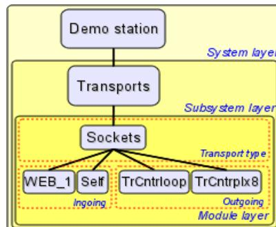
Fig. 6. The layered structure of the transports subsystem.
