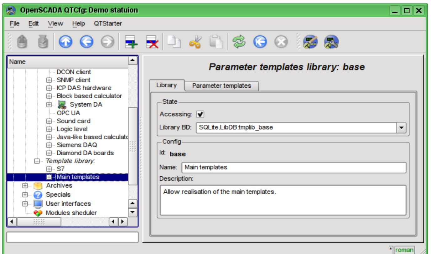
Fig. 4.5d. The main tab of configuration of template library of subsystem "Data acquisition".
